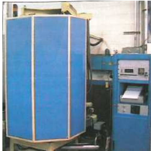
Figure 3 - A unique characteristic of Parker's manufacturing capabilities is our in-house plasma nitriding equipment
